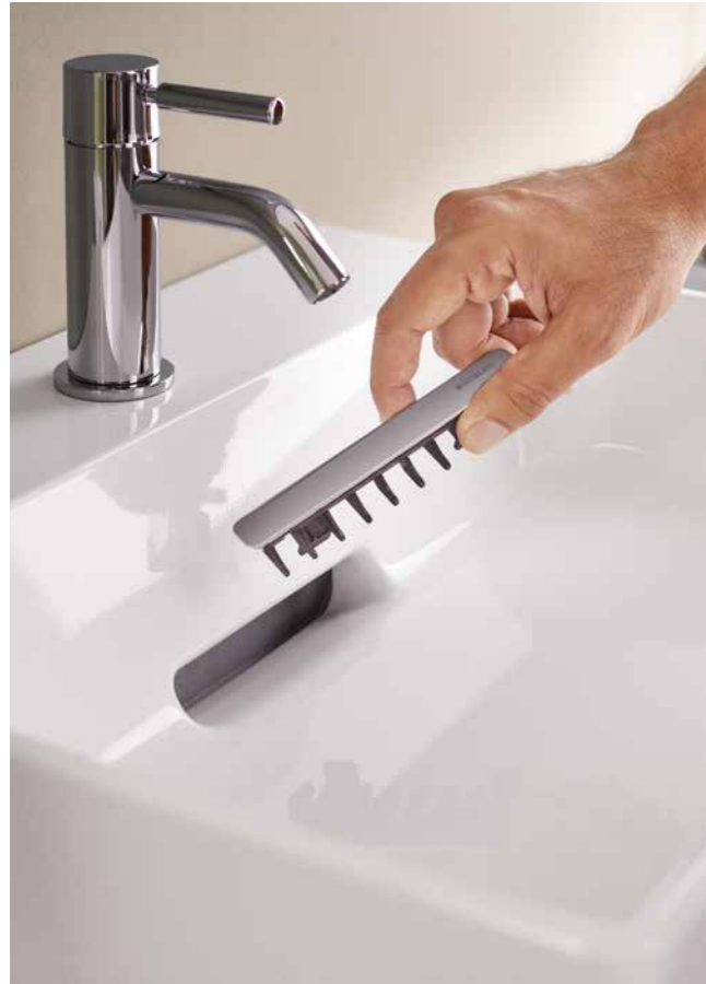
↑ The horizontal drain cover is fitted with a comb insert that stops hair from entering and clogging the trap and drainage system. A magnet holds the cover perfectly in position. The comb insert behind the cover is easy to remove and clean.
